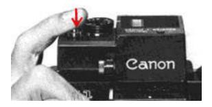
12. When exposure ends, the shutter release button returns to its former position.
