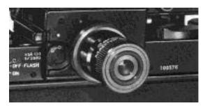
The Canon Magnifier can be attached to the eyepiece. It magnifies the rangefinder section for accurate focusing. Because it can be swung up and clamped, the entire field of view can be viewed after focusing.
