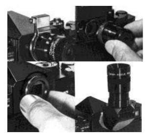
This is an attachable magnifier which serves for precision focusing in close-up photography, copying, and wide-angle photography. With this magnifier, the center of the field of view can be seen with a magnification of 2.5X. It can be fixed on the eyepiece by means of the eyepiece ring. Since not all of the field of view can be seen with the magnifier attached, it is raised on its hinges to make the whole field of view visible through the viewfinder. However, since it cannot be raised up
