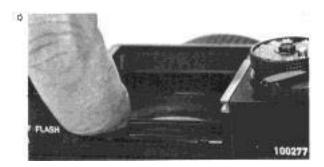
To remove the focusing screen, first detach the pentaprism and insert your finger
