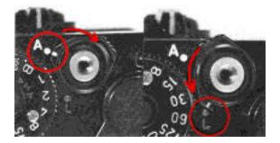
When the mark on the lock ring is not turned to the "A" position, it is impossible to proceed to press the shutter release button or to wind film. This device is useful when carrying the camera around. Shutter release button lock should be turned to-the "L" position to avoid accidental tripping of the shutter.
