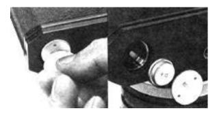
This is the camera's power source for exposure metering. The battery chamber can be opened by unscrewing it with a coin. Be sure to place the battery with the (+) and the (-) poles in the correct position. A new battery will work for about a year.
