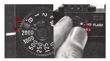
When you set the film speed scale, lift and turn the corresponding ring around the shutter speed dial. To set the dial at a shutter speed of 1/2000 of a second, turn it clockwise until it stops and cannot be turned any more.
