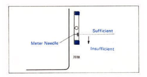
Set the ASA film speed scale at ASA 100 and the. shutter speed at 1/2000 of a second. Then check the position of the meter needle in the viewfinder while at the same time you turn the switch of the power source battery to "C".
